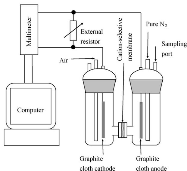
Fig. 1. Schematic of the experimental set-up. Organic substrate is oxidized in the anodic compartment and electrons were transferred via an external resistor to the cathode. The voltage output was measured continuously by a high impedance multimeter.
